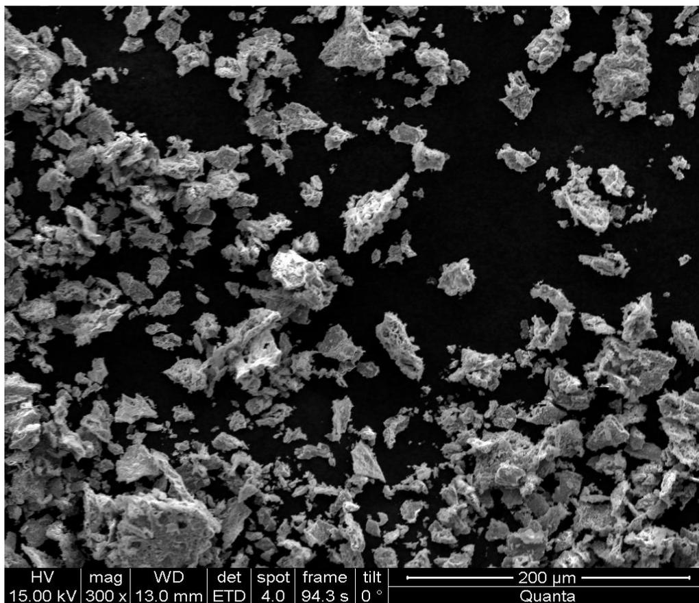
**Figure 2.2:** Scanning Electron Micrograph of the silver nanoparticles used in this work.
