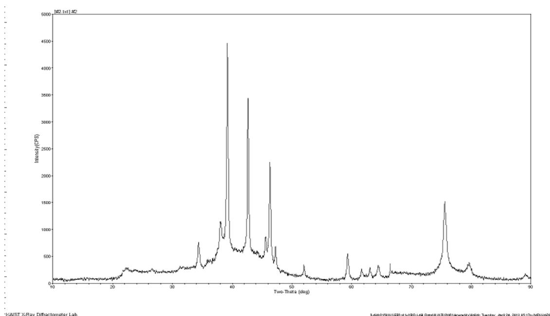
Figure 2.4: X-ray diffraction pattern of Ag-NP at room temperature synthesized by 4-amino-5-benzyl-2,4-dihydro-3H-1,2,4-triazole-3-thione extract with AgNO<sub>3</sub> solution.
