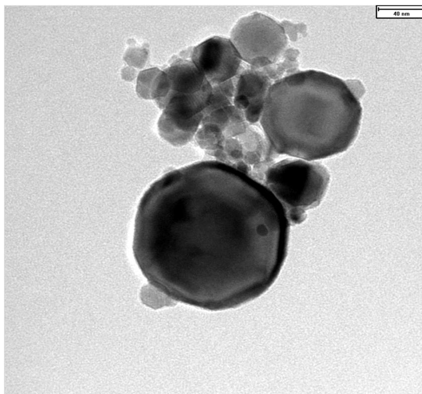
**Figure 2.3:** Transmission electron micrographs of the silver nanoparticles used in this work. (a) The bar marker represents 40 nm, (b) 10 nm
